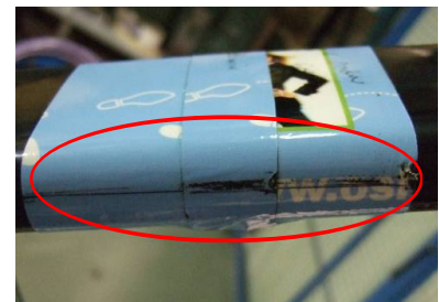
Photo 6 - Film contact / damage
