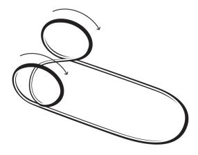
4. Place first coil flat, align inner handrail section and set second coil on top.
