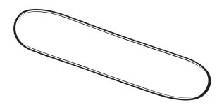
3. Roll handrail creating two separate coils. Be sure handrail is wound neatly on top of itself.
